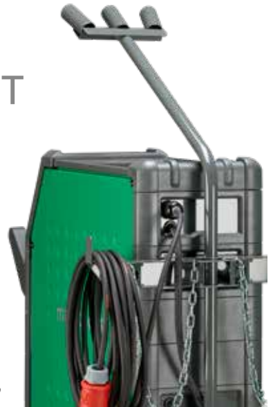
Device for easy coil-up of long cables.
